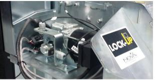
Sealed magnetic proximity sensors with direct drive gear motor
