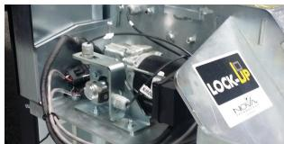
Sealed magnetic proximity sensors with direct drive gear motor
