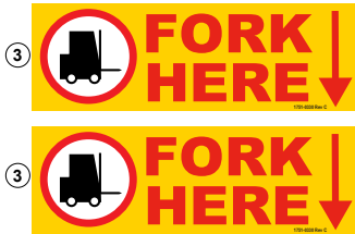
1751-0330 Two positions one on top of each fork pocket.
